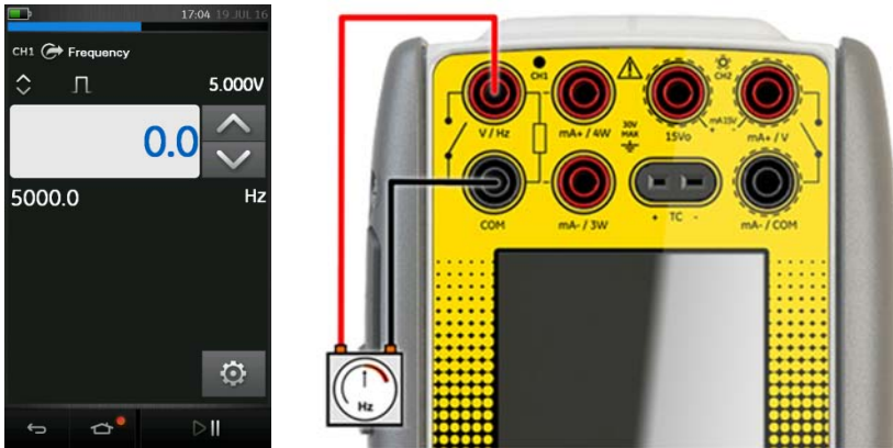
Figure 2-22 Source Frequency CH1 (Range 0 to 5 kHz, Waveform: Square, Amplitude 5.0V)
