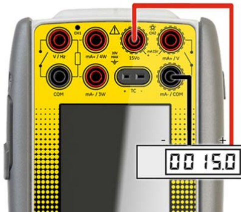
Figure 2-15 Connection Details for 15Vo Unregulated Current Loop Output
