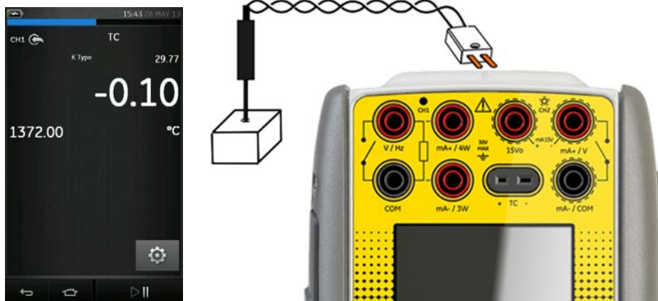
Figure 2-27 K-Type Thermocouple Measure CH1 (Range -270 to 1372 °C)
