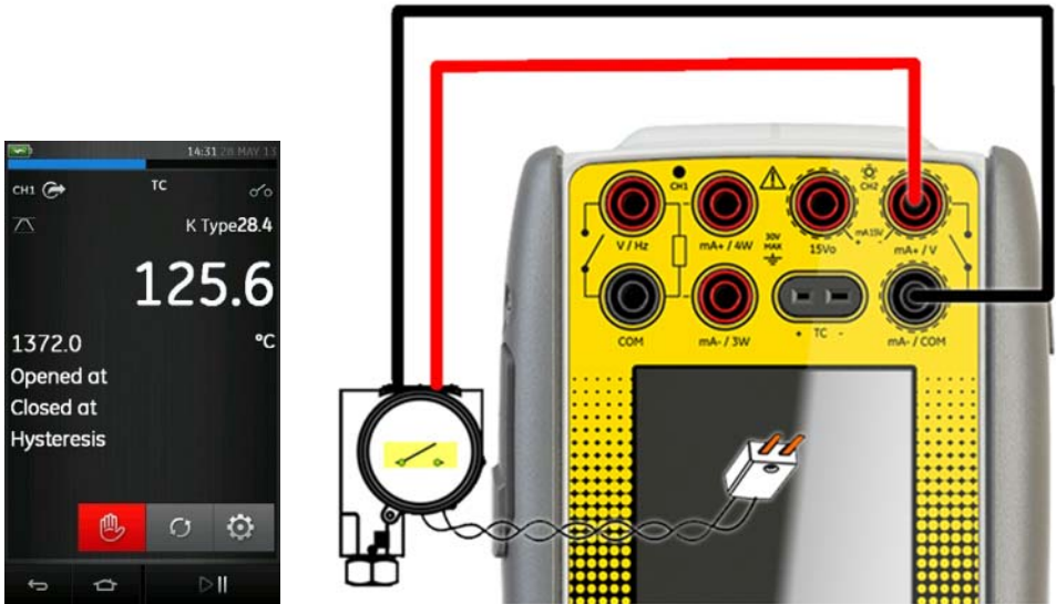
Figure 2-29 CH1 Thermocouple Source, CH2 Switch Test
