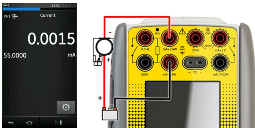
Figure 2-13 Measure Current on CH1, Range \pm 55 mA
