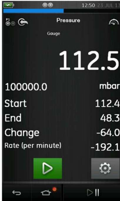
Figure 3-10 Leak Test Example
