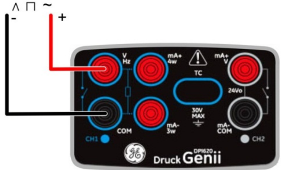
Figure 2-17 Example A - Measure Frequency on CH1 (Range 0 to 50 kHz)
