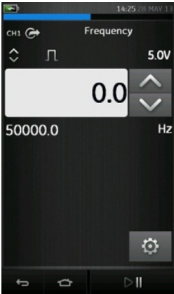
Figure 2-18 Example B - Source Frequency CH1 (Range 0 to 50 kHz)
