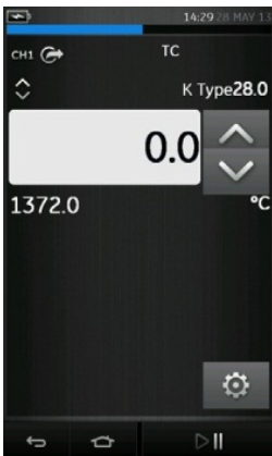
Figure 2-22 Figure 2 21K-TypeThermocouple Source CH1 (Range -270 to 1372 °C)
