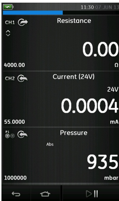
Figure 2-8 Calibrator Window – Reduced View
