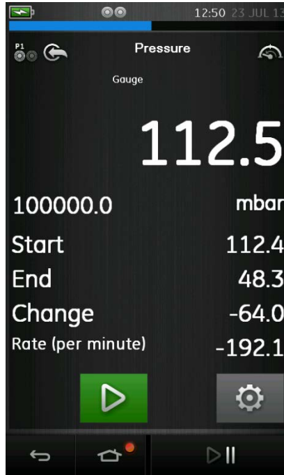
Figure 3-7 Leak Test Example
